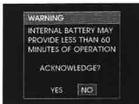
Figure 2 Battery Test Fail Message
